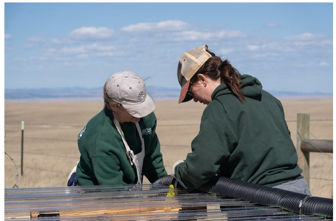
Above photo: rainout shelter designed to mimic drought conditions by capturing a portion of rainfall received at the site. Lower photo: researchers Amy Symstad, USGS (left), and Jacqueline Ott, USFS (right), constructing rain capture system designed to mimic drought conditions. Photos by Erika Reiter, USDA.
